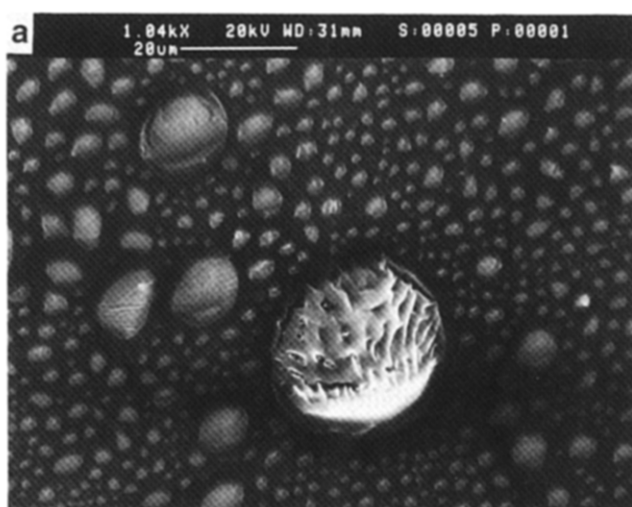
Figure 4 SEM photograph of unmodified silicone rubber
