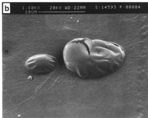
Figure 5 SEM photographs of cross-sections of modified silicone rubber: (a) general view and (b) a bulge fractured by the electron beam
